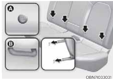
[A]: ISOFIX Anchorage Position Indicator, [B]: ISOFIX Anchorage
